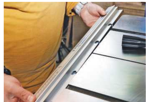
▲ The fence rail removes easily for blade swapping
